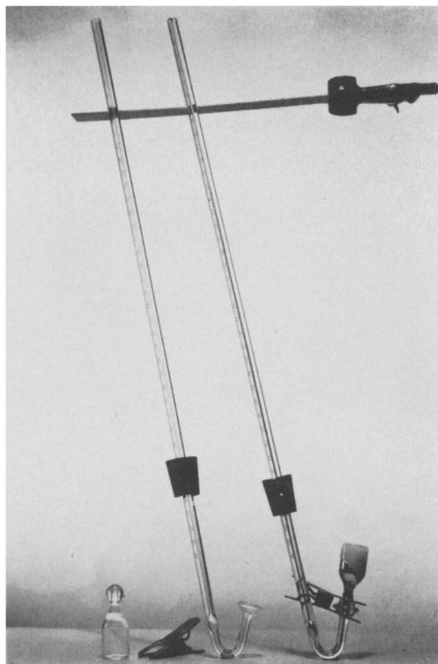
Fig. 1. Picture of unassembled and assembled filled dilatometers.
